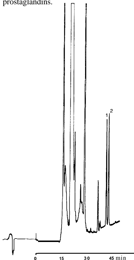
Fig. 4. Separation of two derivatized prostaglandins. Continuous gradient, 65–100% acetonitrile in water (1% acetic acid), Column, 1 m \times 240 \mu m I.D. fused-silica capillary packed with 5- \mu m ODS particles. Peaks: 1 = \text{PGA}_1 ; 2 = \text{PGE}_1 .
